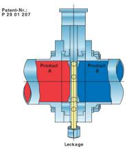
The combination of a double sealing system and a pressure free leakage chamber ensures separation of incompatible fluids.
