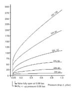
This diagram shows the flow characteristics depending on the pressure drop
