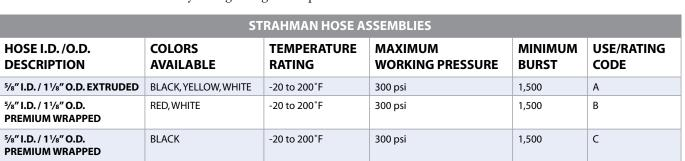
Note: When used with mixing-unit hose stations, the maximum pressure rating will be 150 psi.
