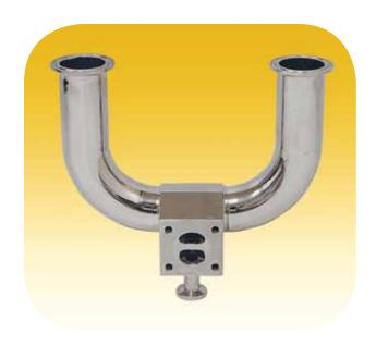
The **Zero DL® Point-of-Use Valve** utilizes the T-pattern design to promote efficient installation when used on clean water loops. The main valve body is machined from a solid block of 316L stainless steel. It's design improves drainability and eliminates deadlegs within a processing system. Available in valve sizes 1/2" to 4" with tubing run sizes through 6" in clamp, buttweld ends, and other specialty connections.
