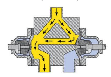
The flow pattern on the closed side of the valve will allow for a continuous flow to the open side providing zero deadleg.
