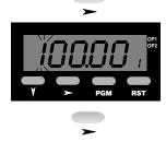
To change the Alarm value, press the Scroll Key. If there was no key activity for 3 seconds, the Alarm value will appear (one digit description shown on secondary display); however, press the Scroll Key in order to edit. The unit will now be in Edit Operation as signified by the most significant digit flashing.\*\*
