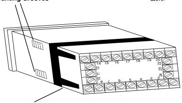
gasket is not distorted and the instrument is positioned squarely against the panel. Slide the mounting clamp into place on the instrument, as shown to the left, and push it forward until it is firmly in contact with the rear face of the mounting panel and the tabs on the bracket arm are seated in the mounting grooves on the side of the unit.
