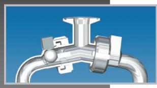
Always a demand for sterile applications: all housing parts of the BIOCOR pumps show no horizontal areas. Each pump comes with four ball lifting magnets, which can be attached to the pump housing from the outside at the location of the four ball valves. The ball valves are risen up magnetically out of their seats and the pump is drained entirely without having to be dismounted. There are no mechanical ball lifters with parts and seals in the wetted area.
