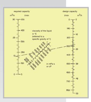
The capacity specified in the pump performance charts generally refer to water (1 mPa $\cdot$ s).
